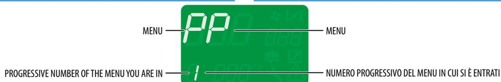
When the compressor is OFF, on the main visualization you enter the main menu to the programming by pushing pay attention, on this way only the menu/parameters without password (level 0) are visible and settable.
