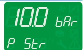
with start pressure value blinking; now you can change the set by and confirm by , so LCD shift to the following: with stop pressure value blinking.
